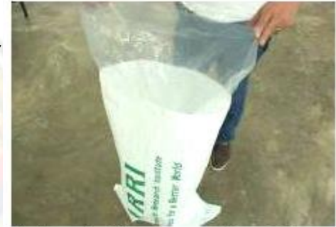
1. Place the Super bag as a liner inside an existing storage bag
