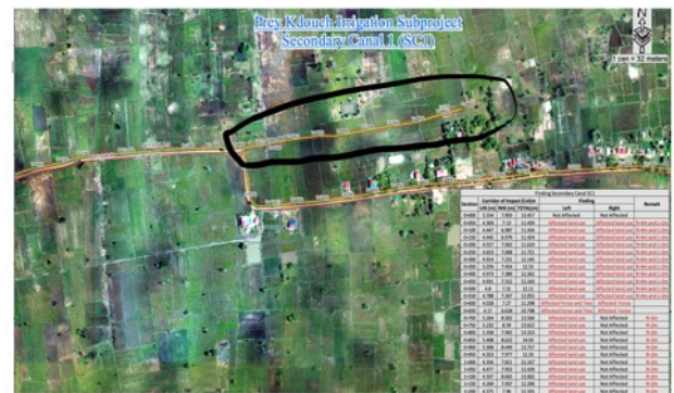
Annex 5: Drone image shows SC1 the new alignment from Pk 1+450 to Pk 1+900
